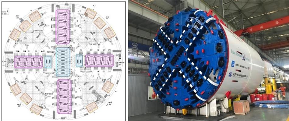
Figure 15. Schematic of the cutterhead (left) and photo of the actual cutterhead (right)
