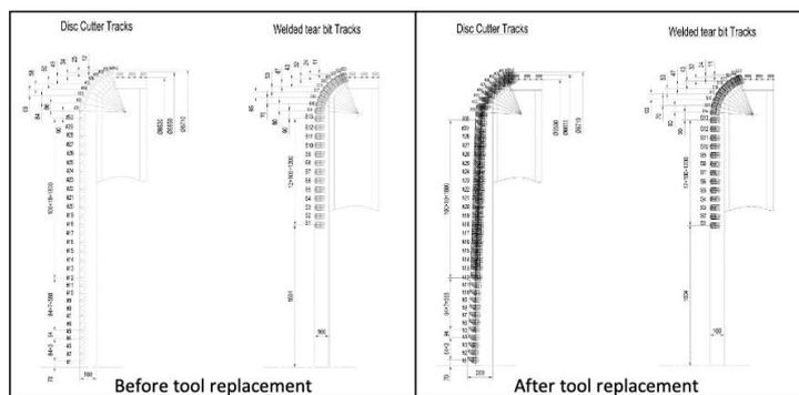
Figure 16. Profile of cutter tracks before (left) and after (right) cutter tools replacement
