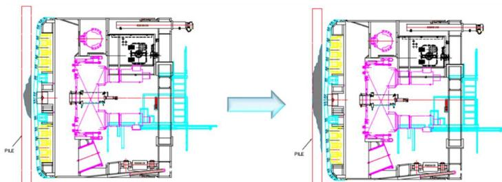
Figure 17. Schematic of the intended approach for the TBM excavating into the piles
