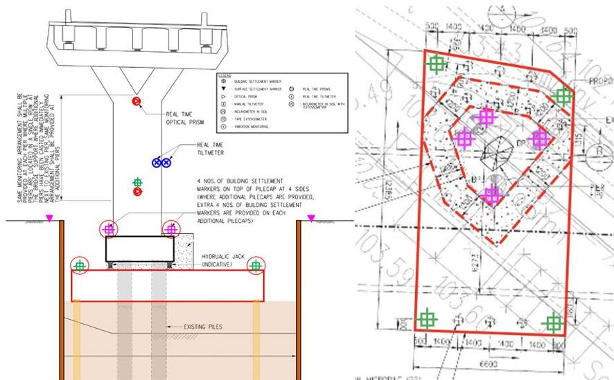
Figure 9. Schematic of the instrumentation layout on the pier in section (left) and plan (right) view
