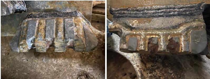
Figure 21. Images of the worn off cutter tools after cutting through the piles
