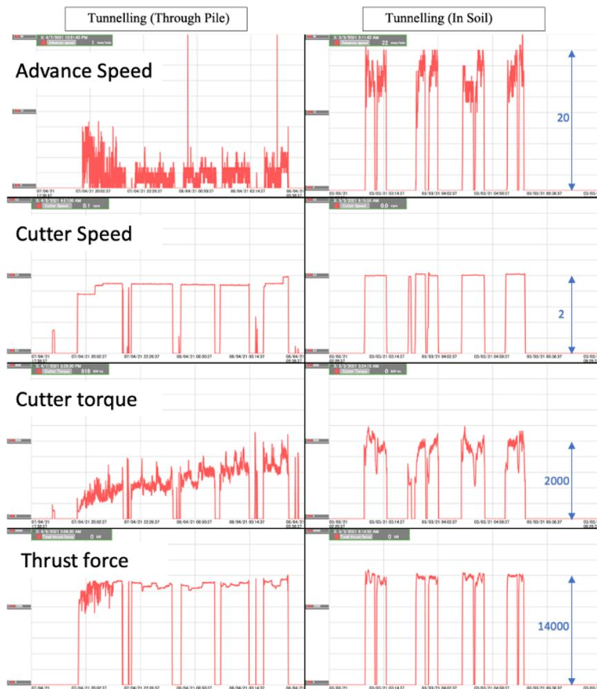
Figure 18. Comparison between the TBM advance speed, cutter speed, cutter torque and thrust force whilst cutting through the pile (left) vs regular tunneling in soil (right)
