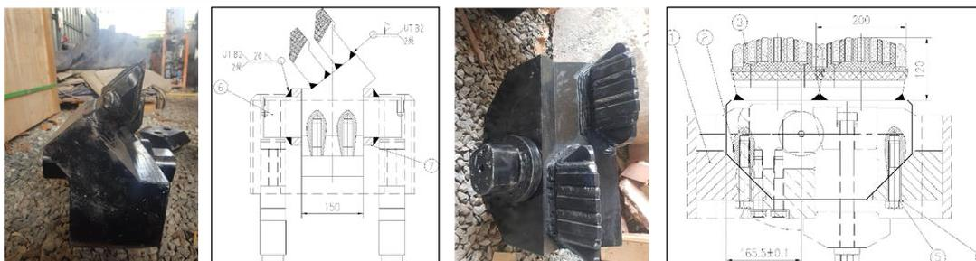
Figure 14. Specialized cutter tools used for pile cutting
