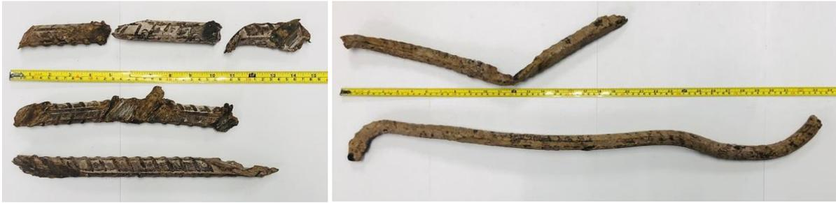
Figure 20. Photos of the rebars retrieved from the excavation chamber after cutting through the piles
