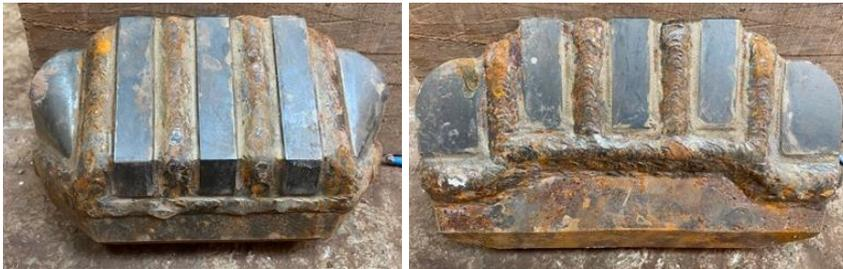
Figure 22. Replacement specialized cutting bits
