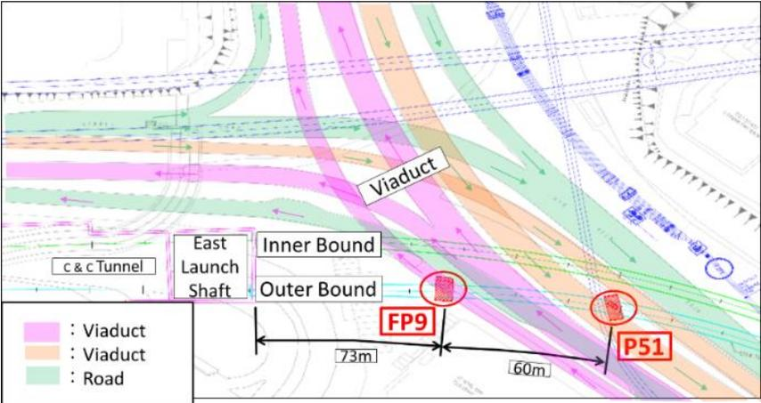
Figure 2. Plan view of the tunnel drives from Keppel Station to Cantonment Station, specifying the piers' location
