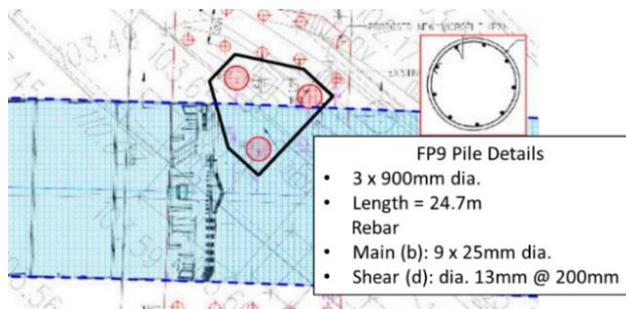
Figure 6. Schematic of the affected piles from plan view
