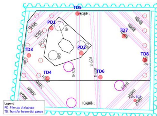
Figure 10. Schematic showing the location of the dial gauges at pier FP9
