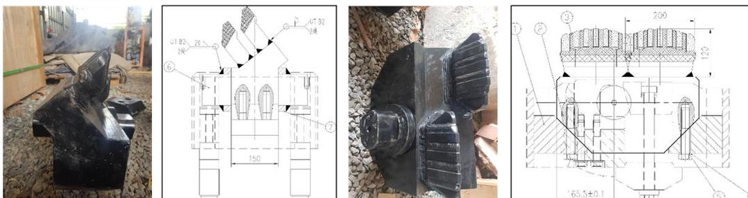
Figure 14. Specialized cutter tools used for pile cutting
