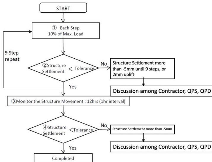
Figure 11. Flowchart depicting the pier jacking procedure
