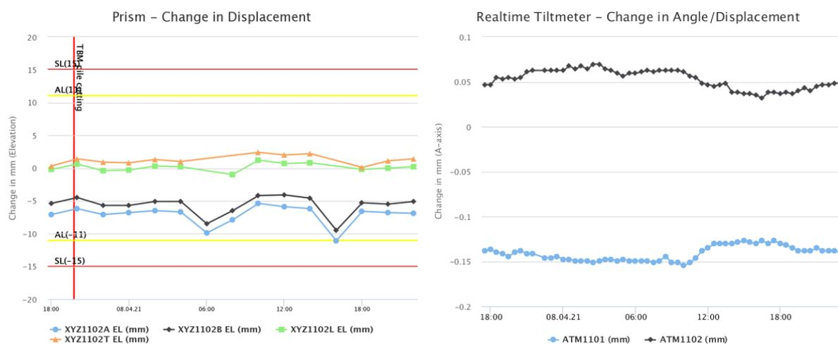
Figure 19. Plots of the real-time optical prisms (left) and tiltmeters (right) during pile cutting
