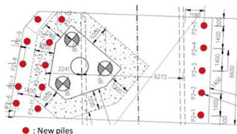
Figure 7. Schematic of the micropiles' location at the transfer beam of pier FP9
