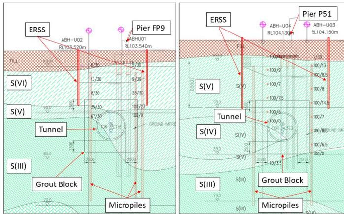
Figure 4. Geological profile at pier FP9 (left) and pier P51 (right)
