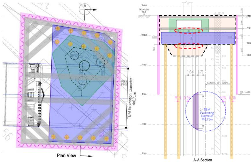
Figure 8. Schematic of the underpinning works in plan and section view
