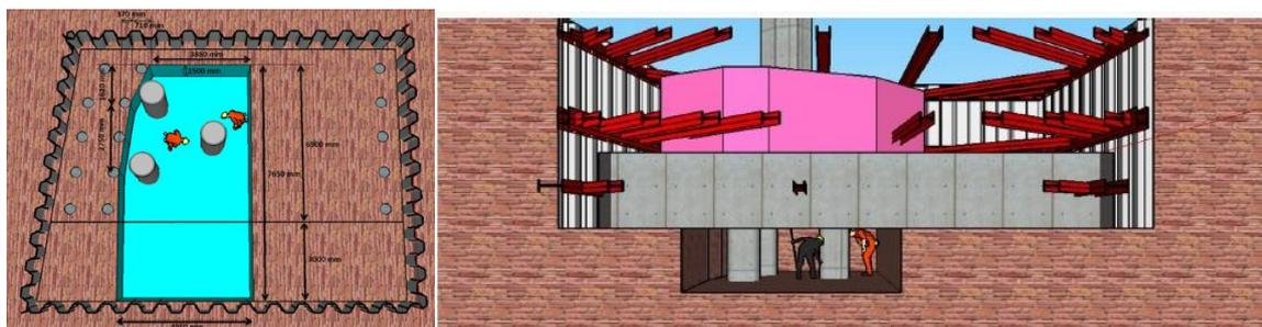
Figure 12. Schematic demonstrating the pile cutting procedure with plan (left) and section (right) views
