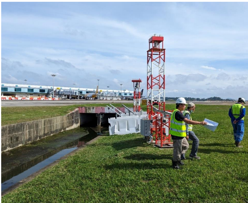
Figure 13: ATS used for reflectorless MOAS grid monitoring.
