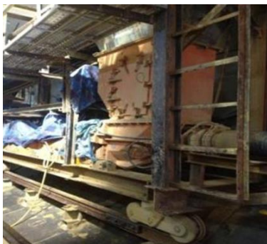
Figure 6. Muckpump Hopper (left) and Snake Pipe Extension (right) on Thomson Line C925
