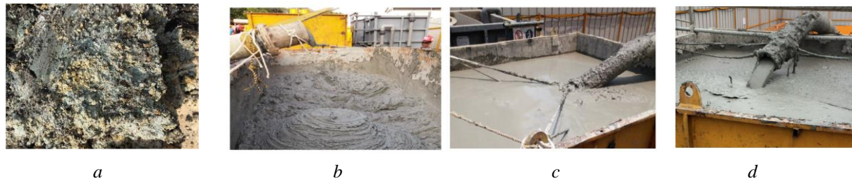
Figure 10. Tests carried out with (a) dry muck with 38% water content, (b) dry muck with 56% water content, (c) wet muck with 105% water content and (d) conditioned muck
