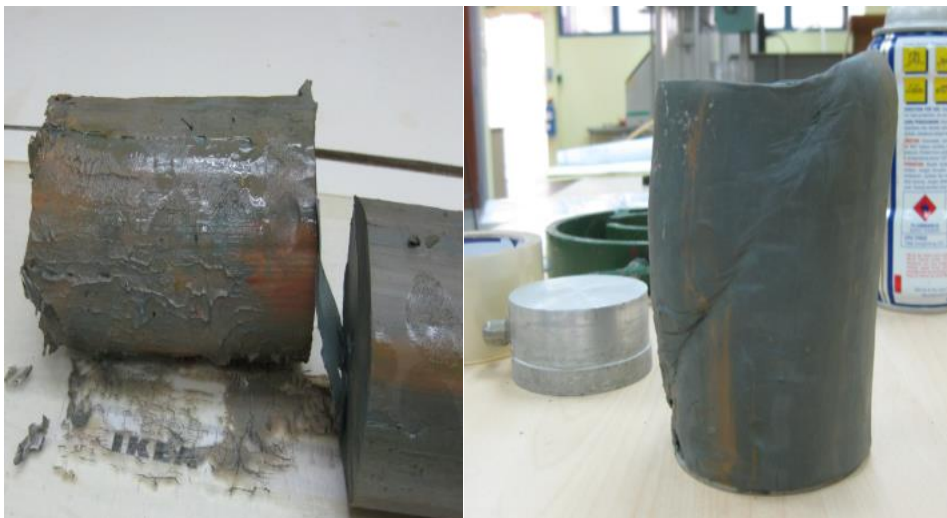
Figure 6 - Sample of Marine Clay of Kallang Formation prepared for triaxial test, showing main representative of soft soil found in Singapore.
