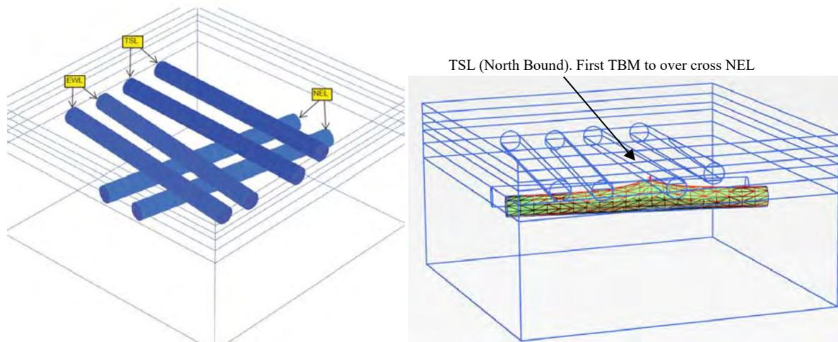
Figure 5. 3D numerical model indicating heave in NEL tunnel due to TSL tunnel excavation
