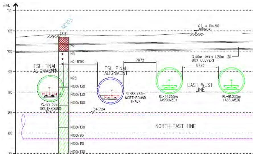
Figure 4. Relative location of tunnels existing tunnels (EWL & NEL) and new tunnels (TSL/T222)
