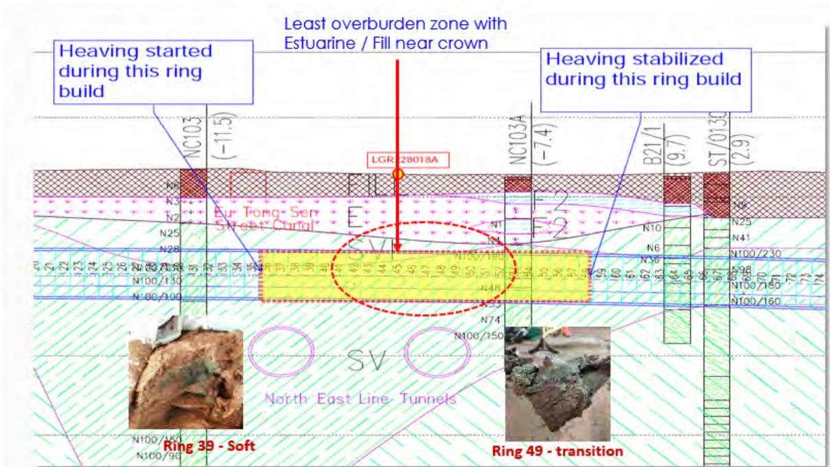
Figure 8. Relative location of existing tunnels, overcrossing TBM tunnel and surface instrument locations
