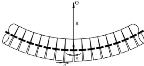
Figure 3. Bending deformation mode of tunnel
