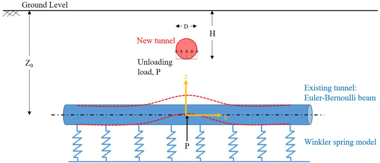
Figure 2. Behaviour of existing tunnel due to overcrossing
