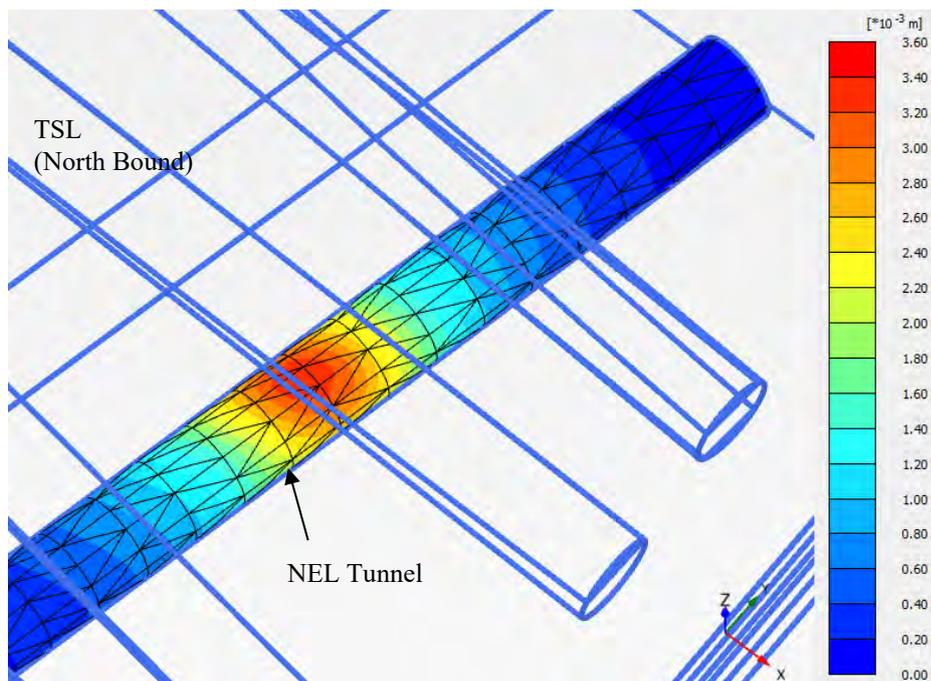
Figure 6. Maximum heave in NEL tunnel due to first TBM overcrossing
