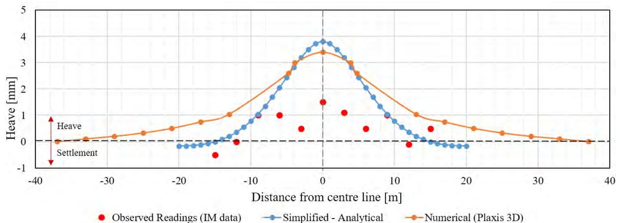
Figure 7. Comparison of numerical estimation, analytical estimation and actual heave readings from site
