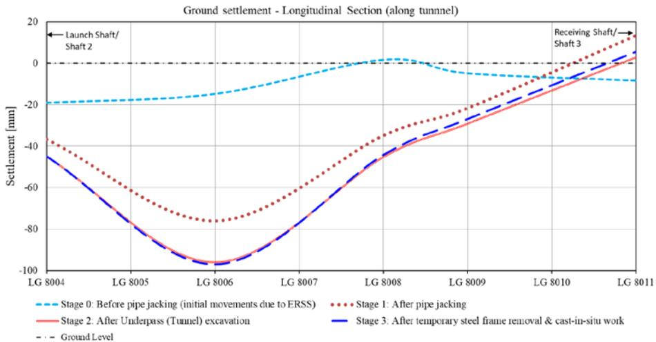
Figure 14: Ground settlement progress during pipe jacking & excavation
