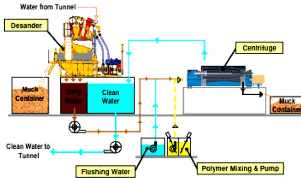
Figure 10: Muck management and slurry treatment system
