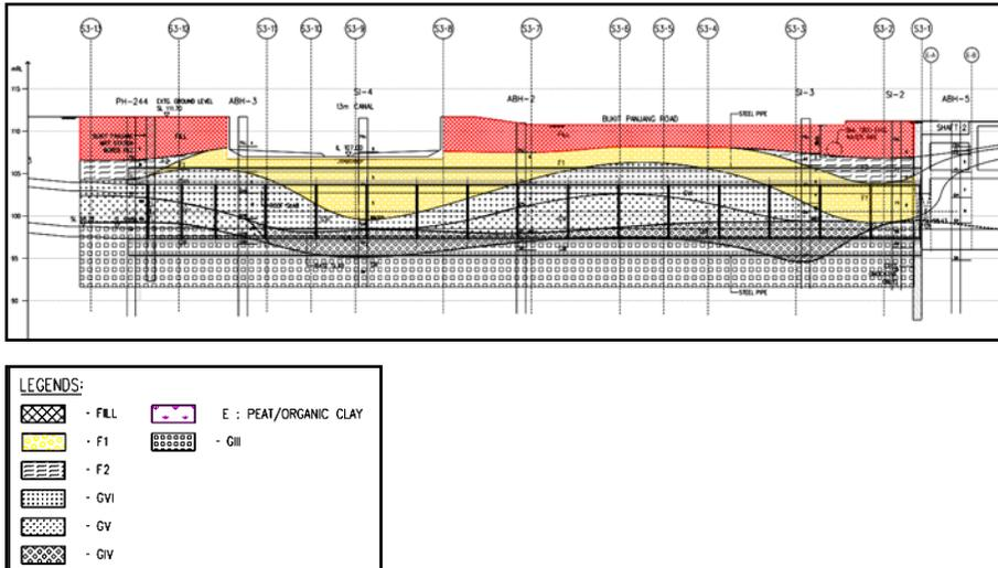
Figure 3: Geological profile along the tunnel
