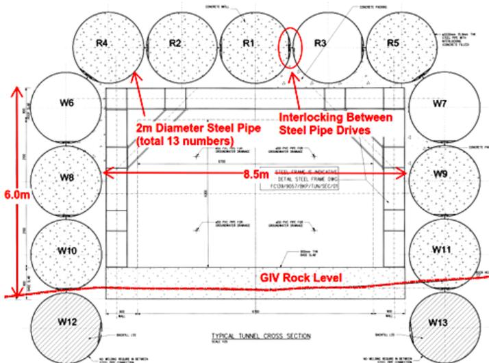
Figure 4: Typical cross section of the linkway
