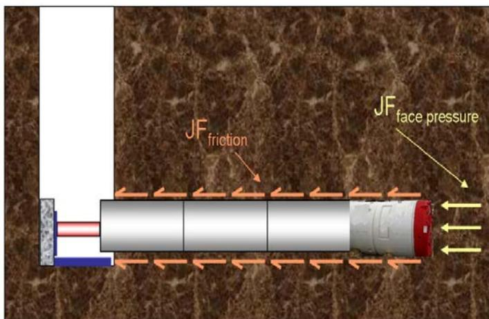
Figure 6: Jacking force estimation
