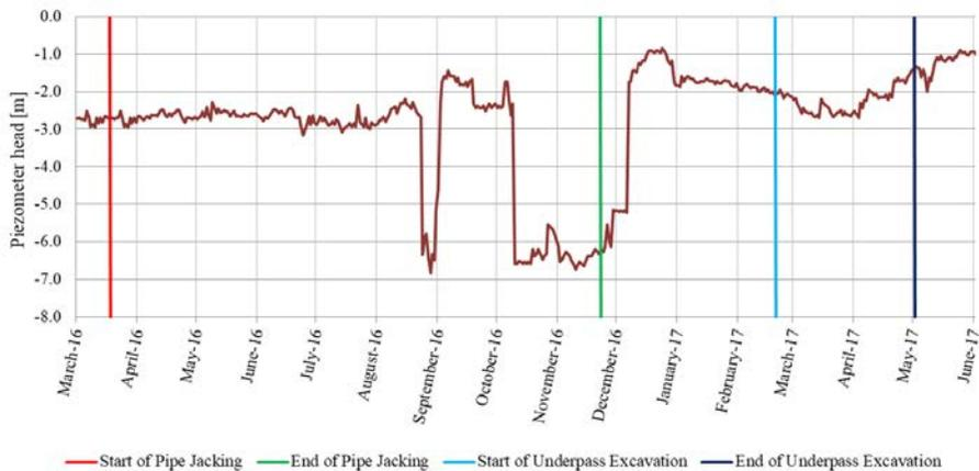
Figure 15: Piezometer Head vs Time
