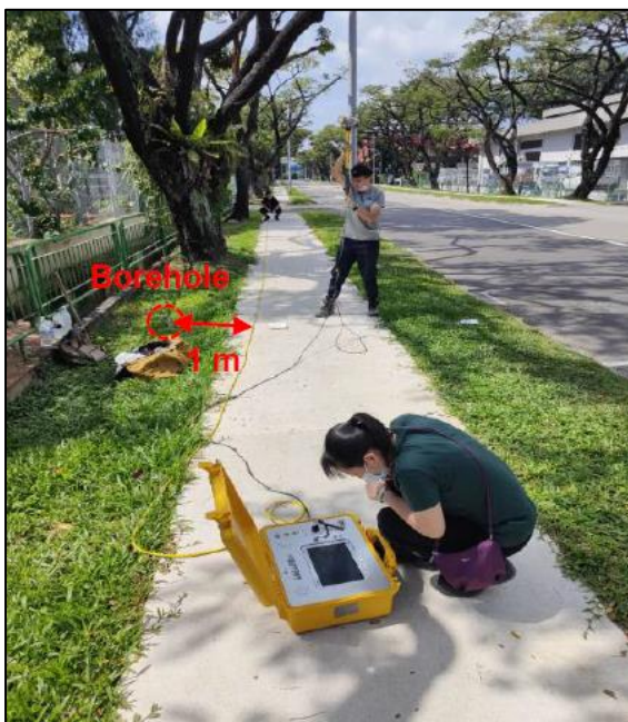
Figure 3.9 Set up of Seismic Scattering with receptors spaced at 1m
