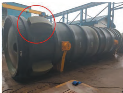
Figure 6. Photo of FRP shaft, highlighting centralizer (red circle) located near the bottom of the shaft.
