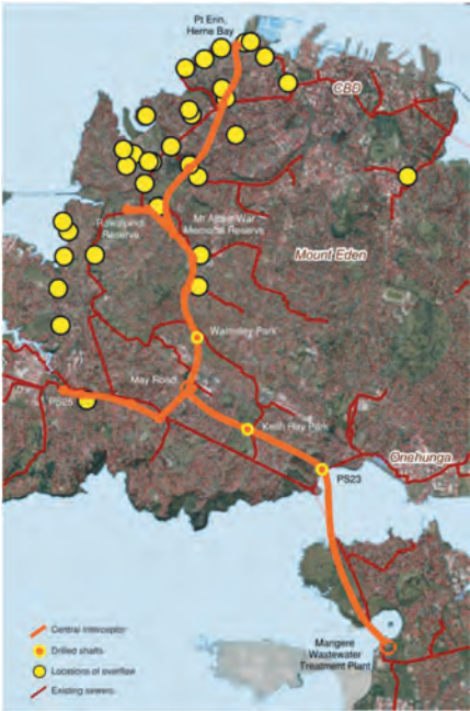
Figure 1. Central interceptor alignment with existing wastewater network and significant overflow locations (Source: Watercare, 2016).
